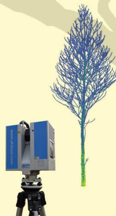
For gathering information about the carbon sequestration potential of trees, Terrestrial laser scanning (TLS) technology is used.
